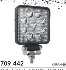
**15W - 2430LM - 9 DIODES - SPOT 30°** 4,3" x 5,1" 10-30 V DC 1,25A@12V / 0,625A@24V
