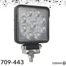
15W - 2430LM - 9 DIODES - FLOOD 90° 4,3" x 5,1" 10-30 V DC 1,25A@12V / 0,625A@24V
