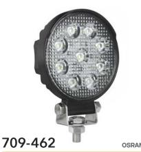
**15W - 2430LM - 9 DIODES - SPOT 30°** 4,2" 10-30 V DC 1,25A@12V / 0,625A@24V
